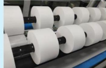
6. Cut off the burrs on both sides, packing in rolls by PE bag and shrinkable film
